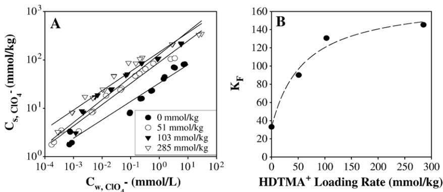
Fig. 3. (A) Freundlich isotherms for perchlorate sorption by SM-SI-GAC at different HDTMA loading rates; (B) dependence of the Freundlich isotherm parameter,  $K_F$ , for perchlorate sorption on SI-GAC modified with different HDTMA loading rates.
