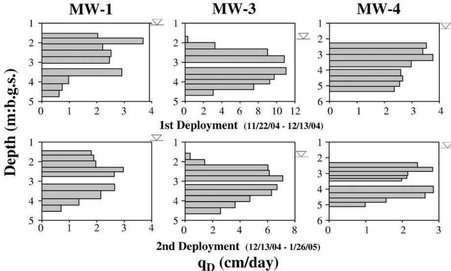
Fig. 7. Comparison of groundwater flux ( $q_D$ ) distributions measured using PFM deployments in MW1, MW3 and MW4 for two time periods at the Indian Head, MD site.
