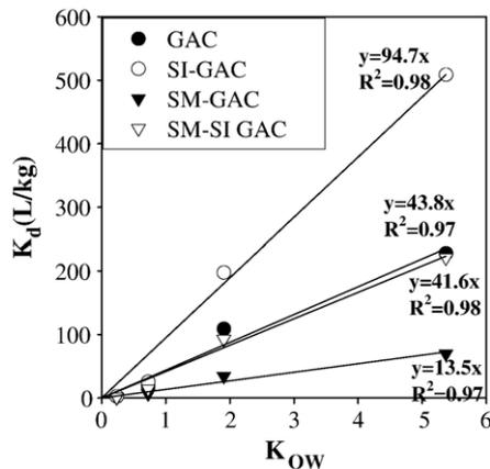
Fig. 5. Correlation of  $K_{ow}$  and  $K_d$  for alcohol sorption by unmodified and surfactant-modified GACs. Solid fitted lines are based on linear regression. The  $K_{ow}$  values are 0.23, 0.72, and 5.4 for methanol, ethanol, and *tert*-butyl alcohol, respectively.
