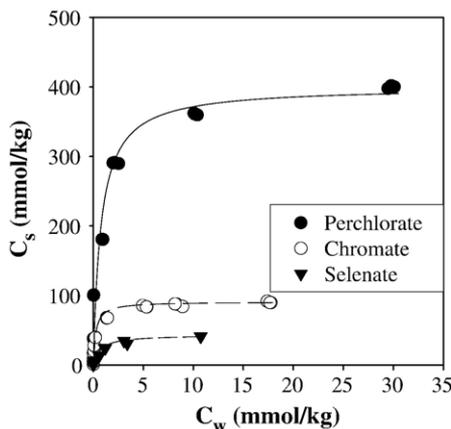
Fig. 4. Sorption of three oxyanions on surfactant-modified GAC (HDTMA-Cl surfactant loading was targeted at 189 mmol/kg). Solid lines are the Langmuir isotherm model fit to the data.
