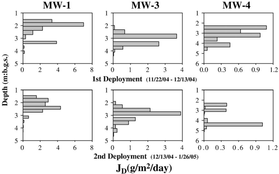
Fig. 8. Comparison of perchlorate flux ( $J_D$ ) distributions measured using PFM deployments in MW1, MW3 and MW4 for two time periods at the Indian Head, MD site.
