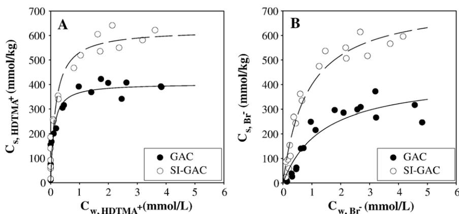
Fig. 2. (A) Isotherms for sorption of HDTMA<sup>+</sup> by GAC and SI-GAC. (B) Isotherms for sorption of Br<sup>-</sup> as a counter ion by GAC and SI-GAC. Solid lines are Langmuir isotherm fits to the measured data.
