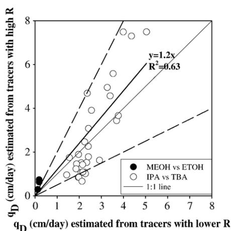
Fig. 6. Comparison of groundwater flux ( $q_D$ , cm/day) values estimated using the depletion of two alcohol tracers during PFM deployments at the Indian Head, MD site. Solid lines representing a 1:1 relationship and linear regression are shown along with dashed lines bounding a factor-of-two deviation from the 1:1 line.
