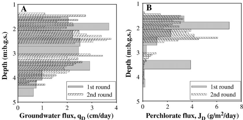
Fig. 9. Comparison of (A) groundwater flux,  $q_D$ , and (B) perchlorate flux,  $J_D$ , distributions determined from PMFs deployed in MW1, with standard sampling (30-cm sections) in the first PFM deployment and high-resolution sampling (5-cm sections) of PMFs for the second deployment.
