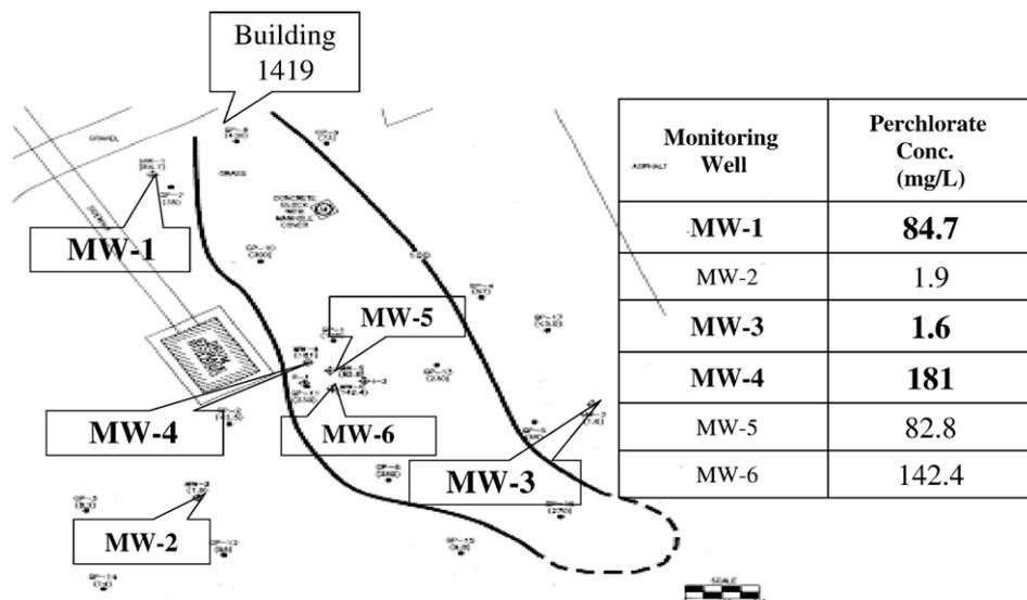
Fig. 1. Perchlorate plume distribution (adapted from Cramer et al., 2004) and location of three monitoring wells (MW1, MW3, and MW4) used for PFM deployments at the Indian Head, Maryland site. Perchlorate concentrations in these and three other wells (MW2, MW5, and MW6), as measured in February 2002 by Cramer et al. (2004), are shown in the inset table. The line is the plume boundary defined by the 100 mg/L perchlorate concentration contour. The scale shown in the figure is 20 feet (~7 m).
